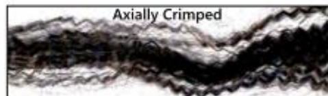
Carbonized rayon filaments (Lee, 1998)
