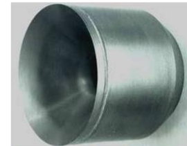
Tungsten throat reinforced with tungsten foam
