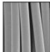
Carbonized PAN filaments (Lee, 1998)
