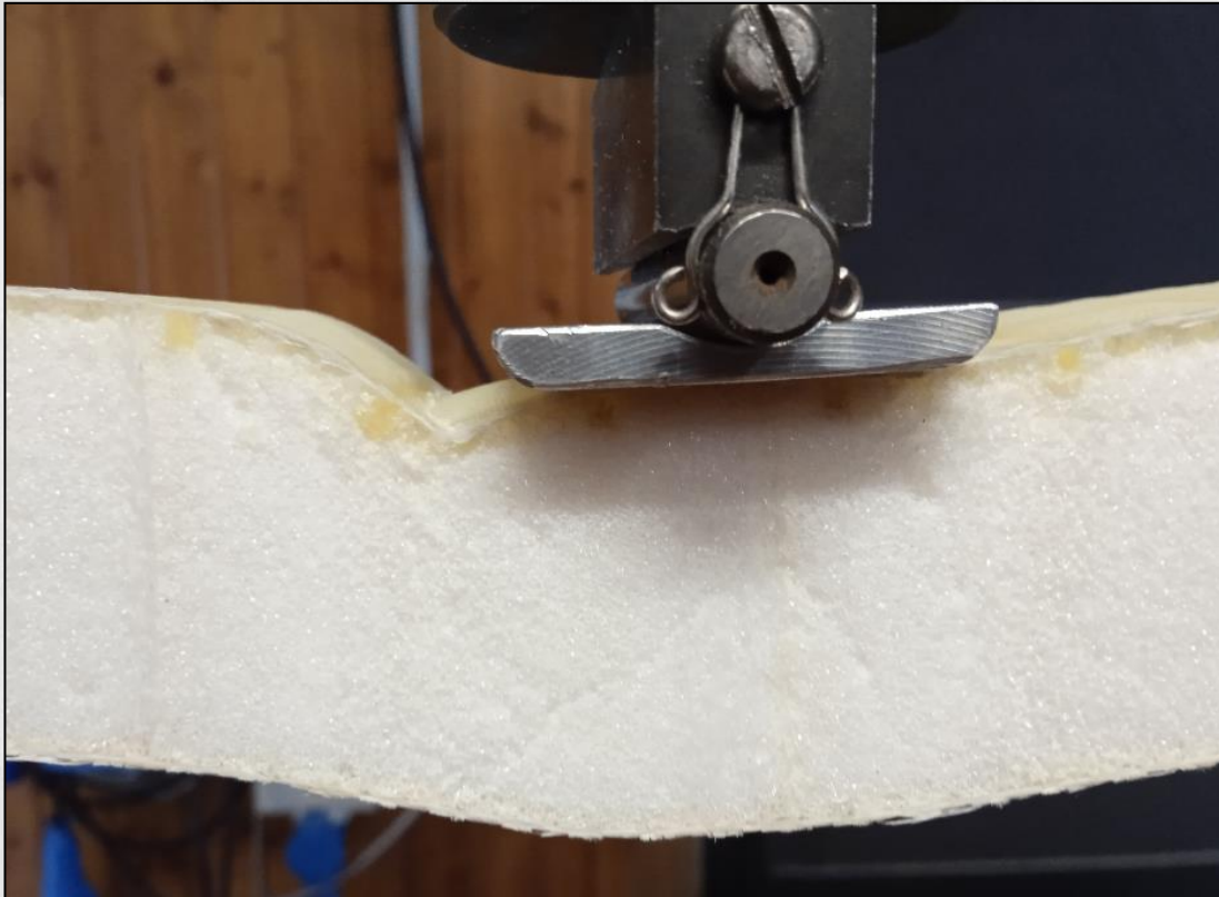
Compression failure under the load point (Skin failure)
