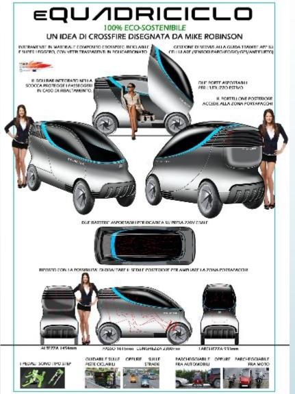
3 Crosspreg® sandwich shells assemble the body 2 Crosspreg® sandwich shells removable doors
