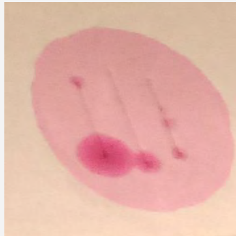
Crease-induced defect (SA-B1) – front side
